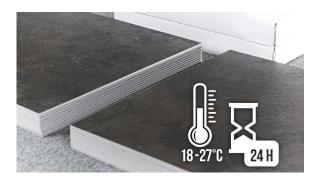
Installations in areas colder than recommended will influence the installation properties of Origin 30 Dryback. The planks or tiles will be less flexible, cutting will be harder and small pieces difficult to cut out. The lower the temperature, the more difficult the installation. Also, the risk to have excessive expansion is increasing with decreasing installation temperature. Installation in areas warmer than recommended increases the risk for excessive shrinking/gaps between panels.
