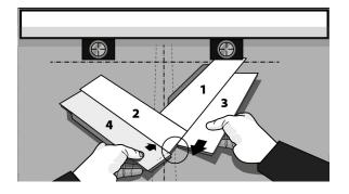
Make sure that the joint is closed tightly. Use hammer and tapping block to gently tap and ensure the locking mechanism is correctly engaged.
