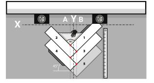
Having placed multiple planks in the centre row. Fill the open triangle close to the wall. Use the spacers to maintain the correct expansion gap between the wall and the floor. It is recommended to place some unopened boxes (or other type of weight) to keep the already installed section in place.
