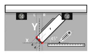
Place your first plank (1). Use another plank (3) and attach it to the first by inserting it into the groove at an angle of +-20°. Do not fold it down. Use plank (3) as a guide to install plank (2). Let plank (3) extend past plank (1) with +-5mm at the bottom. Now insert plank (2) into the short side of plank (1) and slide it till it is stopped by plank (3). Now fold down plank (2).
