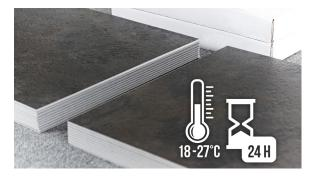
Installations in areas colder than recommended will influence the installation properties of Moduleo<sup>®</sup> Roots. The planks or tiles will be less flexible, cutting will be harder and small pieces difficult to cut out. The lower the temperature, the more difficult the installation. Also, the risk to have excessive expansion is increasing with decreasing installation temperature. Installation in areas warmer than recommended increases the risk for excessive shrinking/gaps between panels.
